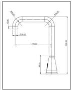
Non-contact self-closing DN 15 Washtable-tap, stainless steel satin; with rotating and lockable angular spout, aerator\*, optosensor.
